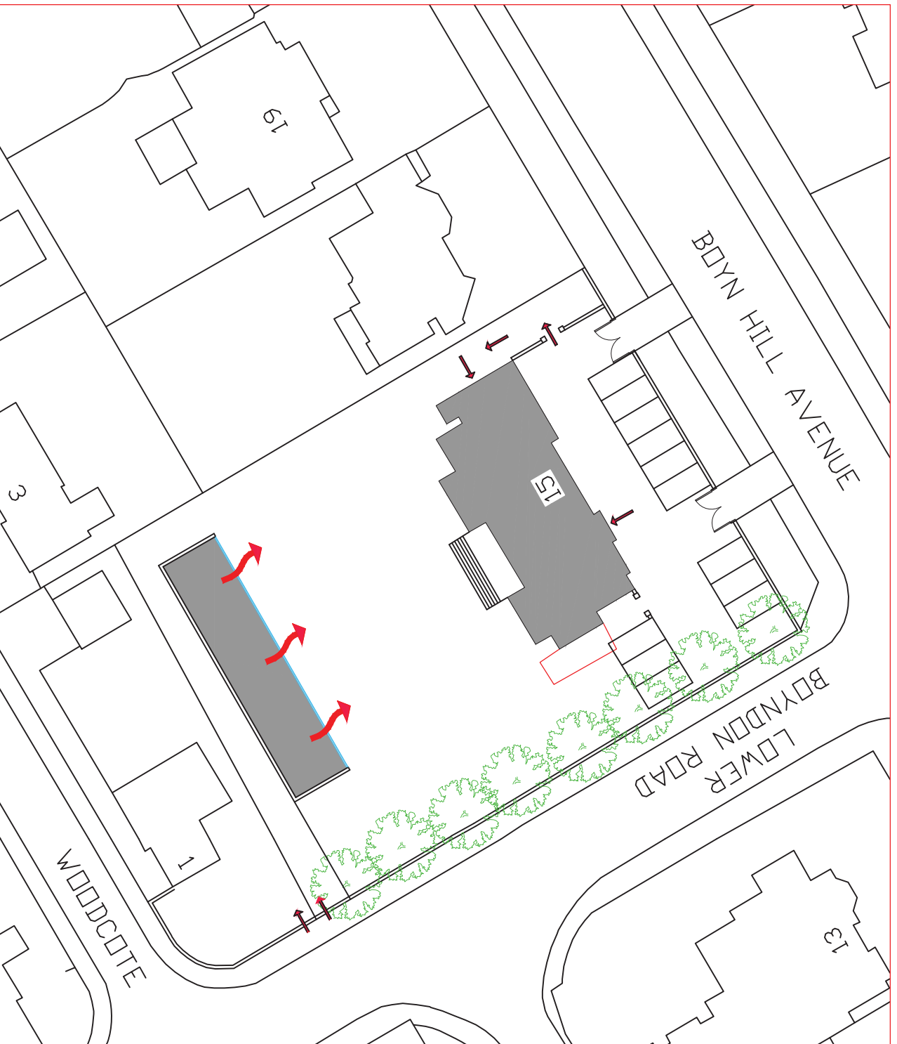
SITE PLAN OPTION 4 - 12 CAR PARKING SPACES - as per option 3. Notional bar/catering facility shown (140sqm) with pedestrian access at rear of garden. Single storey building with glazed facade to garden to allow functions within the garden - associated with marriages at the registry office.
